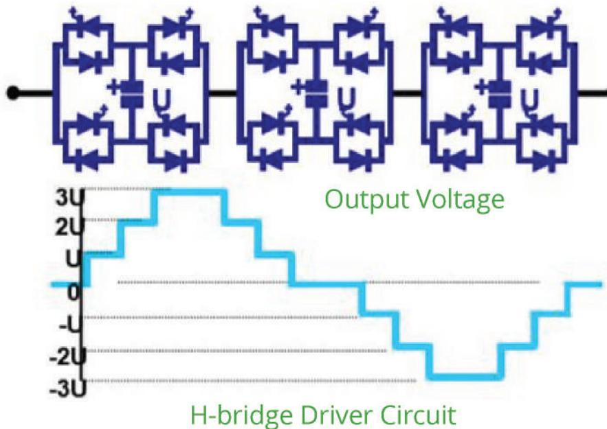
Based on the principle of a voltage source inverter, the RS-SVG uses IGBT (insulated gate bipolar transistors) to control the magnitude and phase of the inverter AC voltage, thus achieving the purpose of reactive power and harmonic compensation. Due to the very high switching frequency of the IGBT (up to dozens of kHz), the SVG can compensate for rapidly changing reactive loads and achieve very high compensation accuracy. SVG is the best solution in the field of reactive power control.
